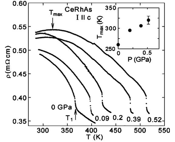
FIG. 2. Electrical resistivity  $\rho_c(T)$  along the  $c$  axis of CeRhAs for  $T > 300 \text{ K}$  under pressures up to 0.51 GPa. Inset shows the pressure dependence of the maximal temperature  $T_{\max}$  in  $\rho_c(T)$ .
