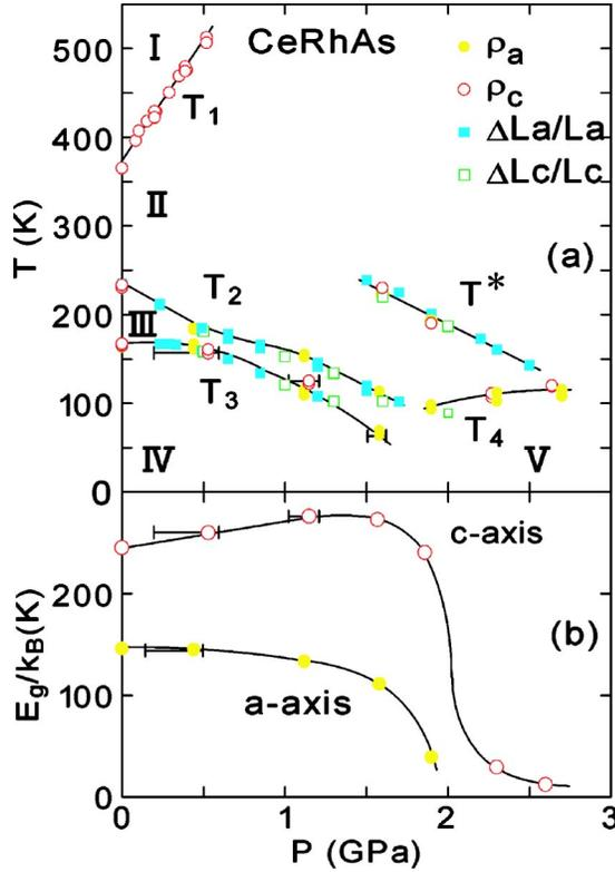
FIG. 1. (Color online) (a) Temperature ( $T$ ) vs pressure ( $P$ ) phase diagram of CeRhAs. Solid lines are a guide to the eye. The phases for  $T \geq T_1$ ,  $T_1 \geq T \geq T_2$ ,  $T_2 \geq T \geq T_3$ ,  $T_3 \geq T$ , and  $T_4 \geq T$  are denoted by I, II, III, IV, and V, respectively. (b) Pressure dependence of the energy gap  $E_g/k_B$ , which is estimated by the activated behavior for  $60 \text{ K} < T < 100 \text{ K}$  in the electrical resistivity for  $I||a$  and  $I||c$ .
