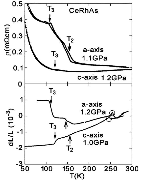
FIG. 9. Temperature dependence of electrical resistivity  $\rho_a$  and  $\rho_c$  and relative length change  $\Delta L_a/L_a$  and  $\Delta L_c/L_c$  of CeRhAs at about 1.1 GPa. The anomalies denoted by circles are due to the freezing of the pressure transmitting medium (Ref. 12).
