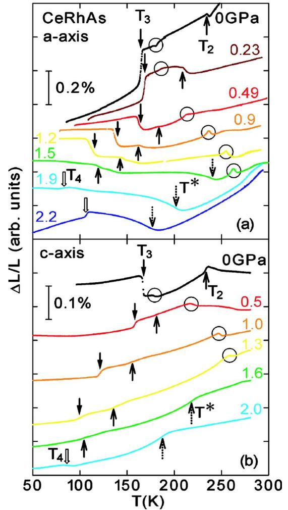
FIG. 6. (Color online) Temperature dependence of relative length change  $\Delta L_a/L_a$  and  $\Delta L_c/L_c$  along the  $a$  and  $c$  axis of CeRhAs under pressures. Data for each pressure are shifted by a constant value for clarity. The anomalies denoted by circles are due to the freezing of the pressure transmitting medium (Ref. 12).
