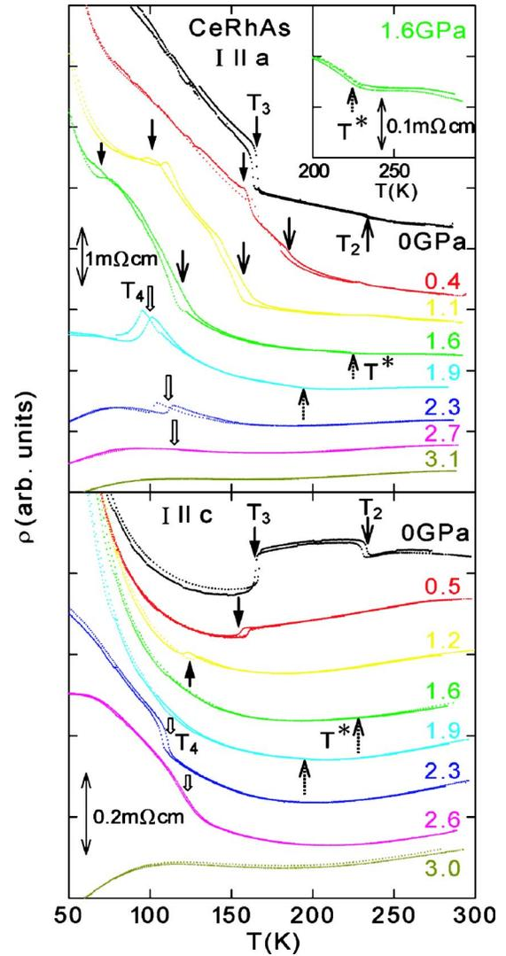
FIG. 4. (Color online) Temperature dependence of electrical resistivity  $\rho_a$  and  $\rho_c$  of CeRhAs for  $50 \leq T \leq 300$  K under pressures. Data for each pressure are shifted by a constant value for clarity. The inset of the upper panel shows up the bend in  $\rho_a(T)$  at  $T^*$ .
