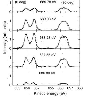
FIG. 2. Doppler profiles of the F\* atomiclike Auger line emitted in the directions parallel and perpendicular to the polarization vector. The spectra are recorded across the F  $1s \rightarrow a_{1g}^*$  resonance of SF<sub>6</sub> for five different photon energies. Baselines are subtracted.
