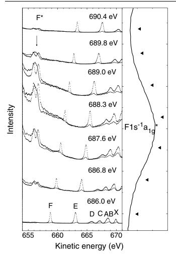
FIG. 1. Electron spectra of SF<sub>6</sub> recorded for parallel (dots) and perpendicular (solid lines) polarizations. The measurements are carried out at seven different photon energies across the F  $1s \rightarrow a_{1g}^*$  resonance, as indicated by the arrows in the right panel, where the total ion yield spectrum is displayed.
