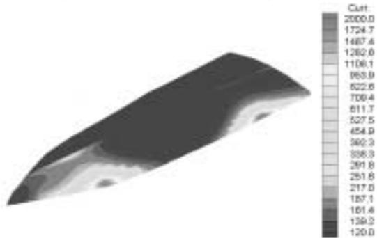
Fig.6 Current density (mA/m<sup>2</sup>) distribution on ship hull surface
