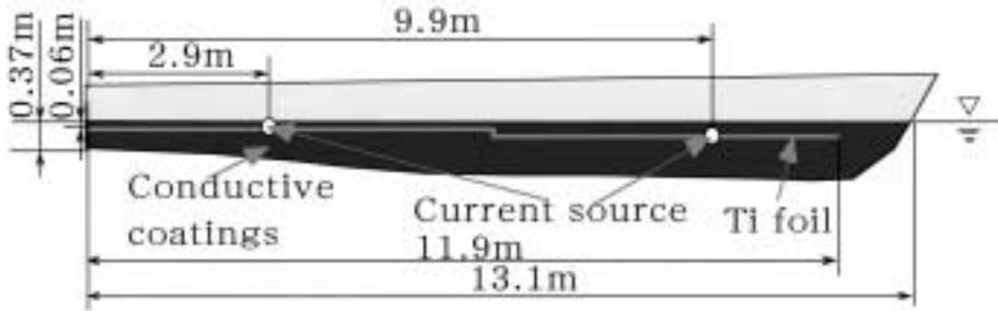
Fig.3 The antifouling system for the passenger boat
