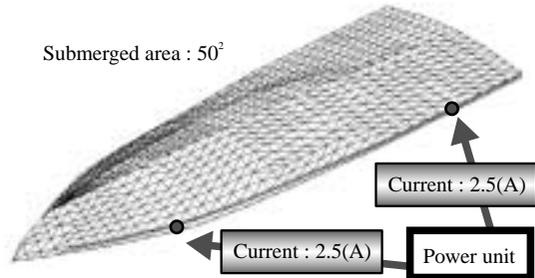
Fig.5 The FEM and BEM coupled model
