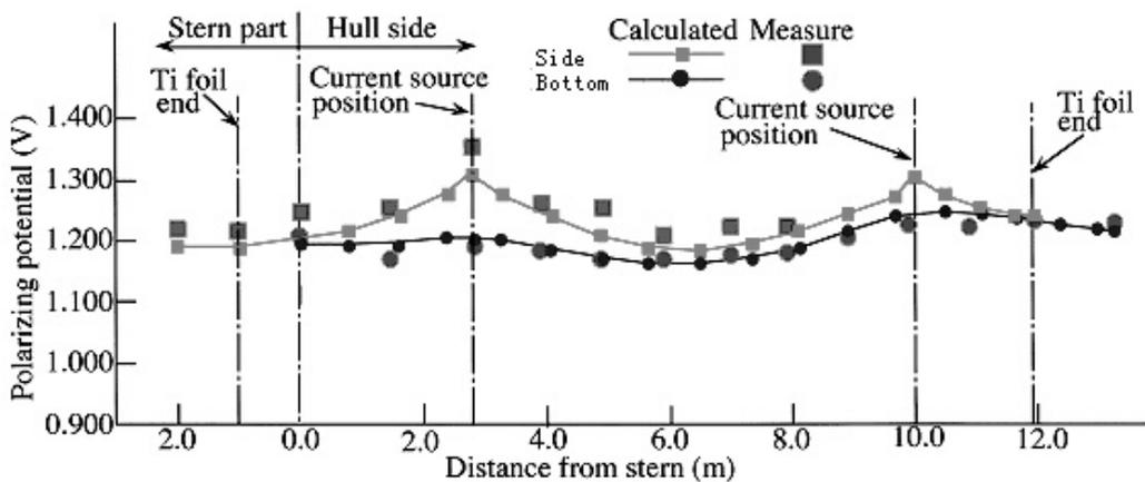
Fig.7 Comparison between calculated and measured potential values on ship hull surface
