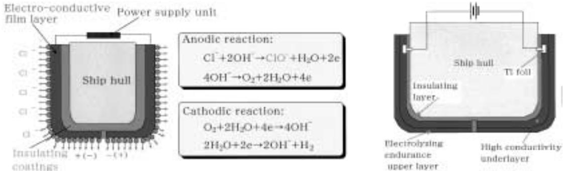
**Fig.1** Principle of the antifouling system applied to a ship hull
