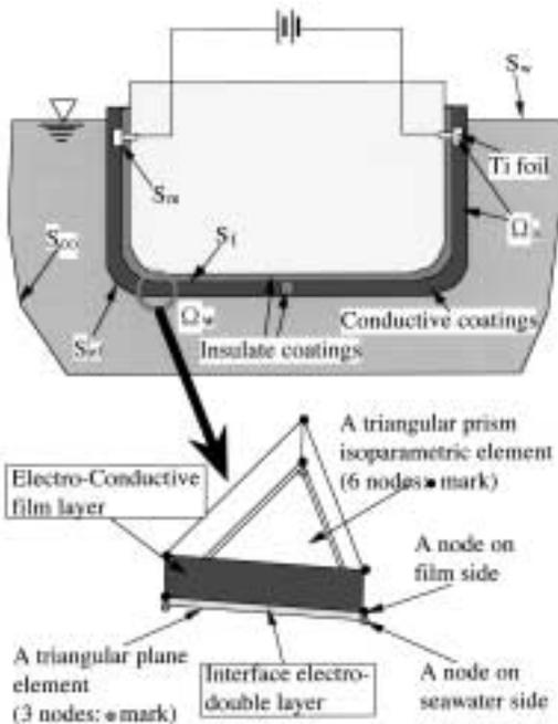
Fig.4 The calculating model for the antifouling system
