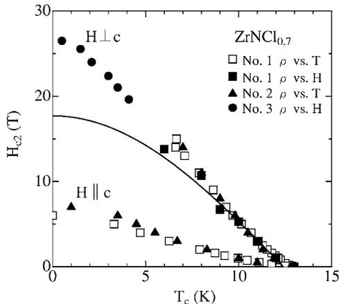
FIG. 5. Temperature dependence of the upper critical field  $H_{c2}$  for  $H \perp c$  and  $H \parallel c$ . The transition temperature  $T_c(H)$  was determined by the 80% level of the normal-state resistivity. The solid line represents the curve calculated using the WHH theory for 3D superconductors (see text).
