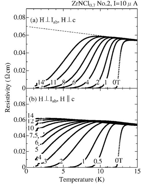
FIG. 3. Temperature dependence of the resistivity of  $\text{ZrNCl}_{0.7}$  for  $H \perp c$  and  $H \parallel c$  for various magnetic fields. The dashed line in (a) represents the linear extrapolation of the normal-state resistivity.
