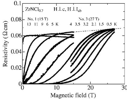
FIG. 4. Magnetoresistance  $\rho(H)$  at selected temperatures. In the  $T$  range of 4–13 K,  $\rho(H)$  was measured for sample No. 1 using a solenoid-type superconducting magnet; in the  $T$  range of 0.5–4 K,  $\rho(H)$  was measured for sample No. 3 using the hybrid magnet. The dashed line in the figure is the line expected from linear extrapolation of the normal-state resistivity in Fig. 3(a).
