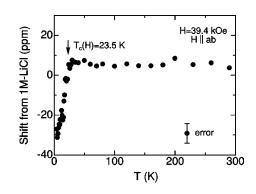
FIG. 5. Temperature dependence of <sup>7</sup>Li-NMR shift at 39.4 kOe for H||ab.
