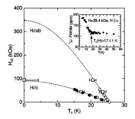
FIG. 4. Temperature (*T*) dependence of the upper critical field  $H_{c2}$  for H||ab and H||c. The mean-field transition temperature  $T_c(H)$  was determined by three methods; 3D LLL scaling ( $\bigcirc$ ), linear extrapolation ( $\bigcirc$ ), and NMR measurement ( $\square$ ). The dashed lines are theoretical curves for the clean limit.<sup>13</sup> Inset shows *T* dependence of the <sup>7</sup>Li-NMR linewidth at 39.4 kOe for H||c.
