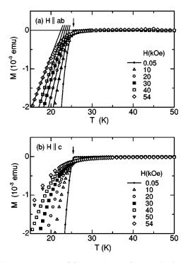
FIG. 2. Temperature (*T*) dependence of magnetization curves for (a) H||ab| and (b) H||c|. Arrow shows  $T_c$  at H=50 Oe. The data were corrected for a *T*-independent background.
