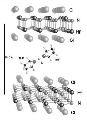
FIG. 1. Schematic structural model of Li<sub>0.48</sub>(THF)<sub>v</sub>HfNCl.
