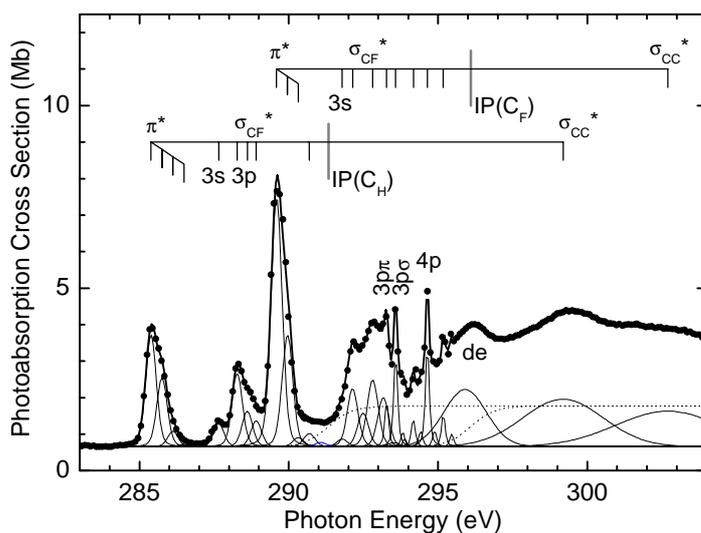
Fig. 1. Total photoabsorption cross-sections of  $CF_2CH_2$  in the C K-shell excitation region. Circles are the experimental data and solid curves are obtained by the least-squares curve fitting. Peak assignments are also given in the figure. The “de” means double excitation.
