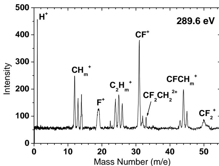
Fig. 2. Linear-TOF mass spectrum observed in the  $C_F$   $1s \rightarrow \pi^*$  transition of  $CF_2CH_2$  at 289.6 eV.
