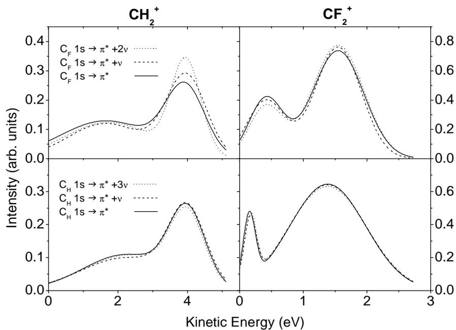
Fig. 3. Kinetic energy distributions of the  $CH_2^+$  and  $CF_2^+$  fragment ions observed by exciting the  $C_F$   $1s$  electron (upper panels) and the  $C_H$   $1s$  electron (lower panels) of  $CF_2CH_2$ .
