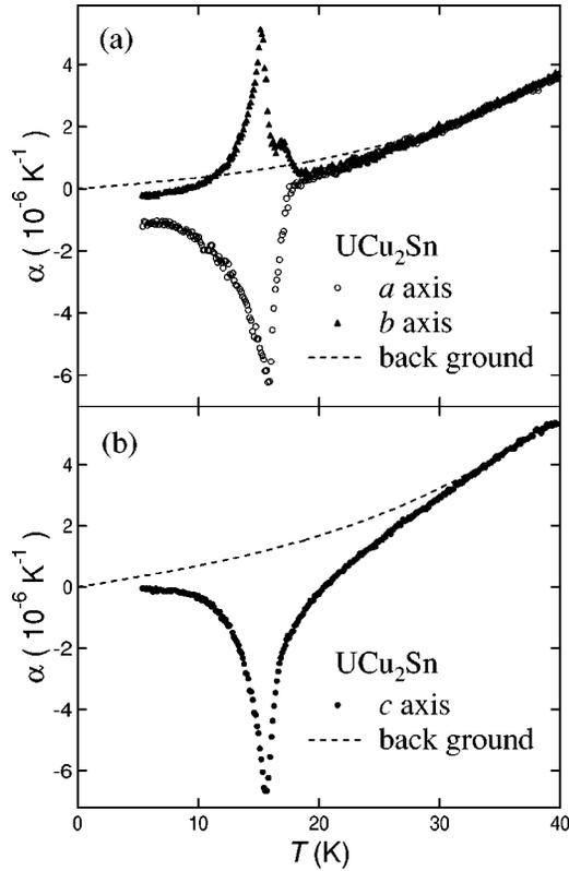
FIG. 5. Temperature dependence of the thermal expansion coefficient  $\alpha(T)$ . (a) Open circles denote  $\alpha$  measured along the  $a$  axis and solid triangles along the  $b$  axis. The broken curve indicates the background  $\alpha_{\text{bg}}$ . (b) Solid circles denotes  $\alpha$  along the  $c$  axis and the broken curve indicates the background.
