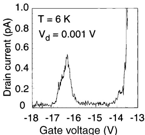
FIG. 3. Drain current vs gate voltage characteristics at  $6$  K (drain voltage  $V_d$  of  $0.001$  V).
