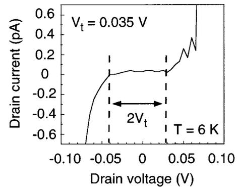
FIG. 4. Drain current vs drain voltage characteristics at  $6$  K (the gate voltage  $V_g$  of  $-14.6$  V).
