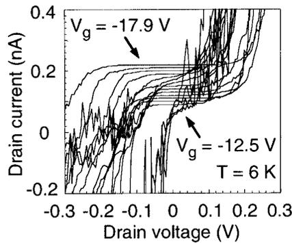
FIG. 2. Drain current vs drain voltage ( $I_d$ - $V_d$ ) characteristics as a function of gate voltage ( $V_g$ ) at 6 K.  $V_g$  from  $-17.9$  to  $-12.5$  V in  $V_g$  steps of  $0.3$  V. The curve for  $V_g$  of  $-13.7$  V is not shown due to measurement failure. Each curve is offset by  $10$  pA per  $0.3$  V of  $V_g$  to provide clarity.
