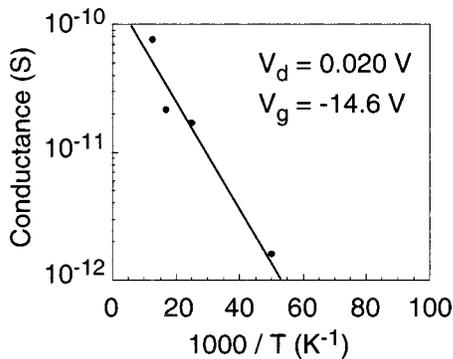
FIG. 5. Arrhenius plot of the conductance at drain voltage  $V_d$  of 0.020 V. The gate voltage  $V_g$  is  $-14.6$  V.
