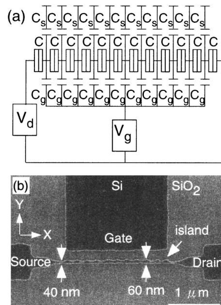
FIG. 1. (a) Equivalent circuit of a fabricated SET with MTJs consisting of 11 islands.  $C_s$ ,  $C_g$ , and  $C$  represent the substrate capacitance, gate capacitance, and tunnel junction capacitance of a Coulomb island, respectively. Parasitic capacitance  $C_0$  of the island consists of  $C_s$  and  $C_g$ . (b) Plan-view scanning electron microscopy micrograph of the SET.
