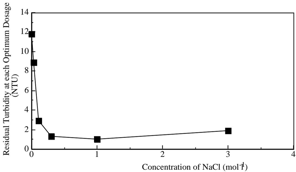
Figure 2. Effect of NaCl concentration on coagulation activity.
