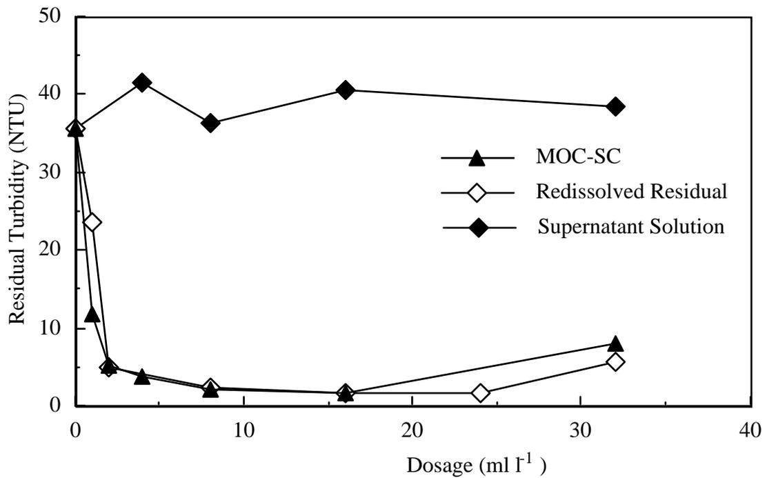
Figure 4. Coagulation using purified extracts of MOC-SC.
