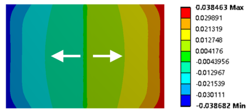
(c) Outdoor opening 0.015 mm (at crack)
