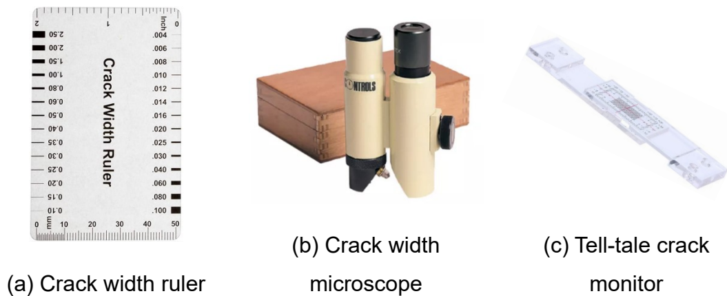
Figure 2–15 Some tools for measuring crack width
