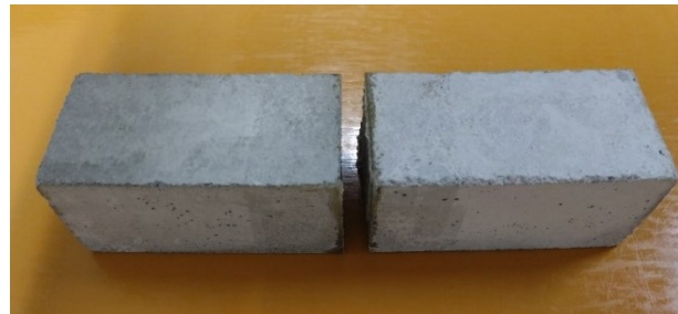
Figure 4–46 Typical damage pattern of HE specimens: Fracture.
