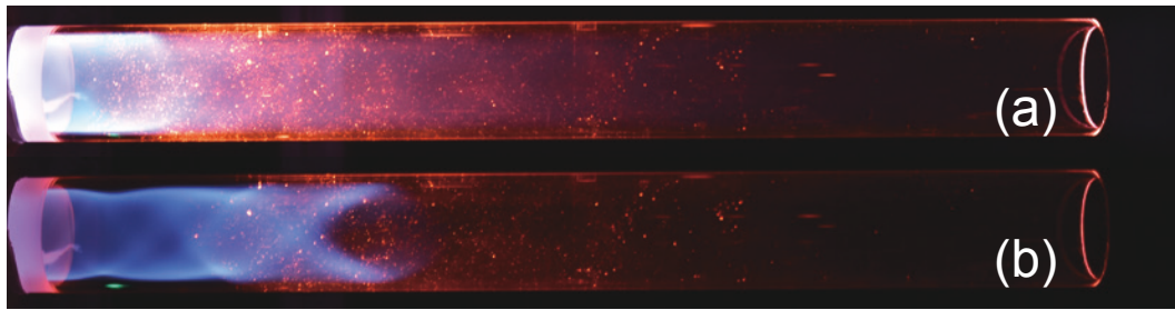
Figure 4.3: Photographic images of the tubular flames obtained using \phi values of (a) 1.0 and (b) 0.59.
