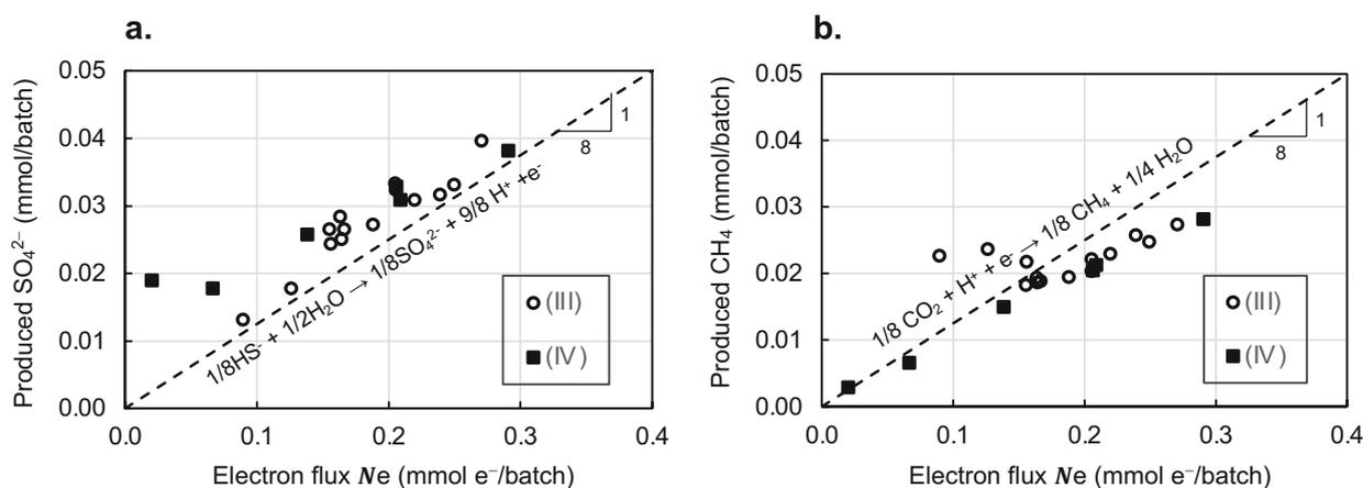
**Fig. 4-6** Produced SO<sub>4</sub><sup>2-</sup> (a) and CH<sub>4</sub> (b) versus electron flux  $N_e$ . Dash lines: theoretical production based on the half reactions.
