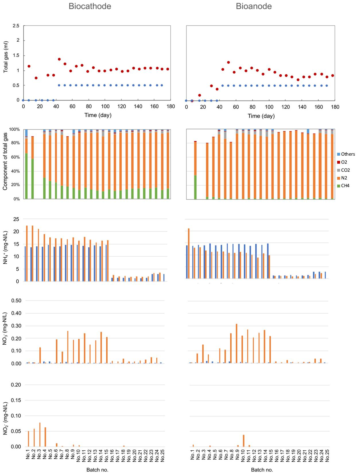
**Fig. 5-4** The measure values (gas components, NH<sub>4</sub><sup>+</sup>, NO<sub>3</sub><sup>-</sup> and NO<sub>2</sub><sup>-</sup> concentration) of RUN
