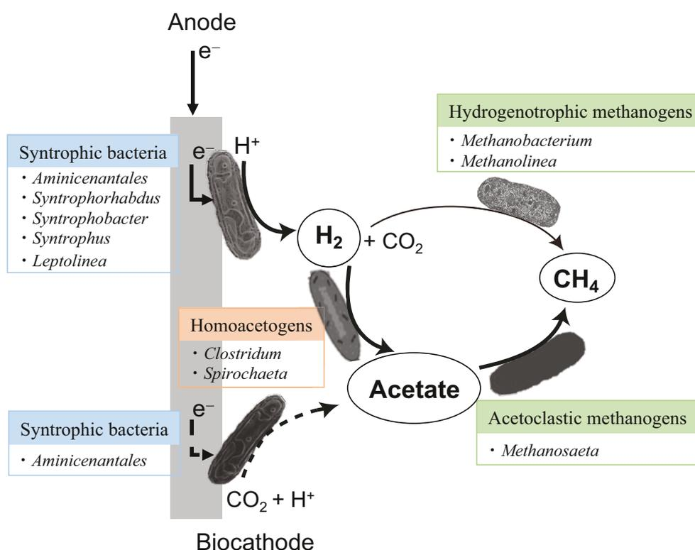
**Fig. 4-8** Scheme of electronic methane production at the biocathode in microbial electrosynthesis system without organic substrates
