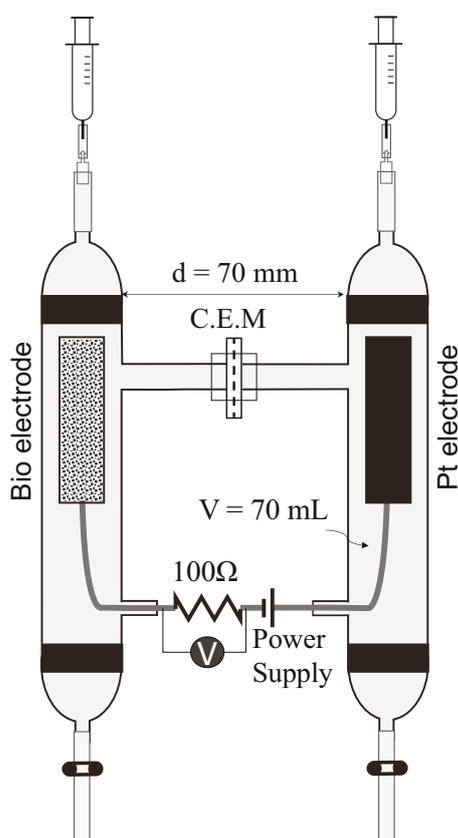
**Fig. 4-1** Schematic representation of microbial electro-synthesis system consisting of two chambers connected with a cation exchange membrane (MES; abiotic anode).
