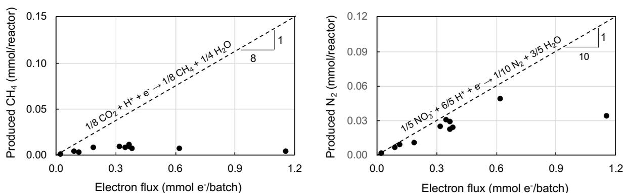
**Fig. 3-9** Produced  $\text{CH}_4$  and  $\text{N}_2$  versus electron flux  $Ne$ . Circle: measured productions, dash lines: theoretical production assuming that all yield electrons  $Ne$  are only used for the reduction of  $\text{CO}_2$  or  $\text{NO}_3^-$ .
