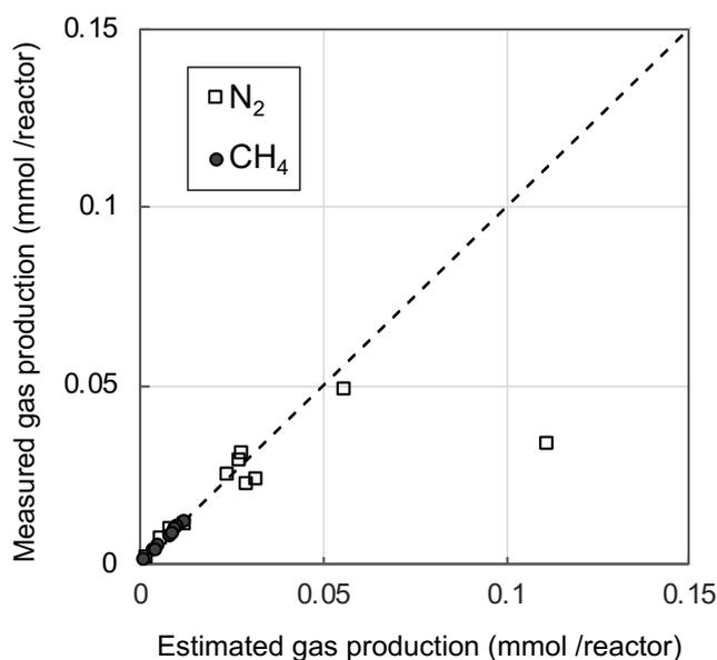
**Fig. 3-11** Comparison between measured and estimated gas production. Estimation of produced CH<sub>4</sub> and N<sub>2</sub> was performed assuming that all electrons  $N_e$  were used for reduction of both CO<sub>2</sub> and NO<sub>3</sub><sup>-</sup>, while electrons from the ratio in Fig. 4 were used for CH<sub>4</sub> production.
