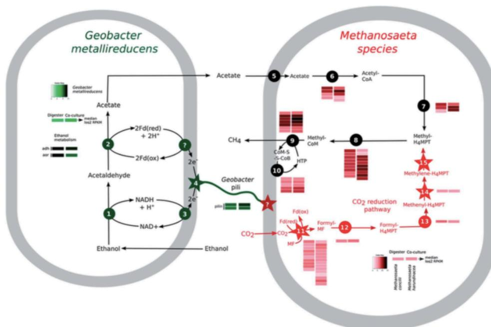
**Fig. 2-4** DIET-based on metabolism in digester samples and defined co-cultures of *Geobacter metallireducens* and *Methanosaeta harundinacea* as revealed metatranscriptomics. (Rotaru *et al.*, 2013)
