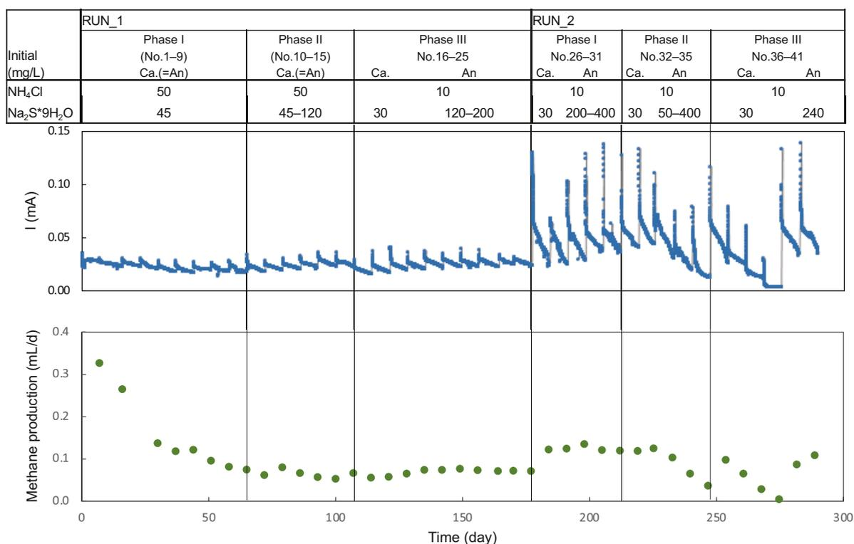
**Fig. 5-2** Batch experiments of microbial electrosynthesis system including RUN 3-1 and RUN 3-2
