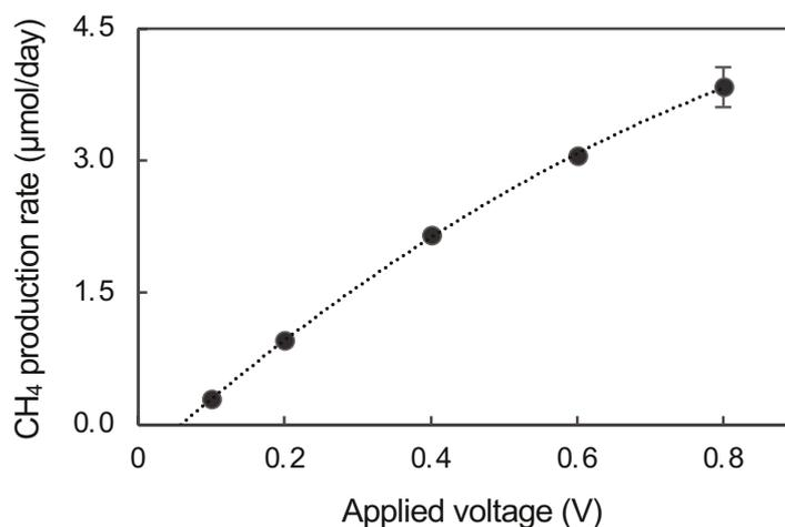
**Fig. 4-5** CH<sub>4</sub> production rates at different applied voltages in phase III (batches 28–29) and phase IV.
