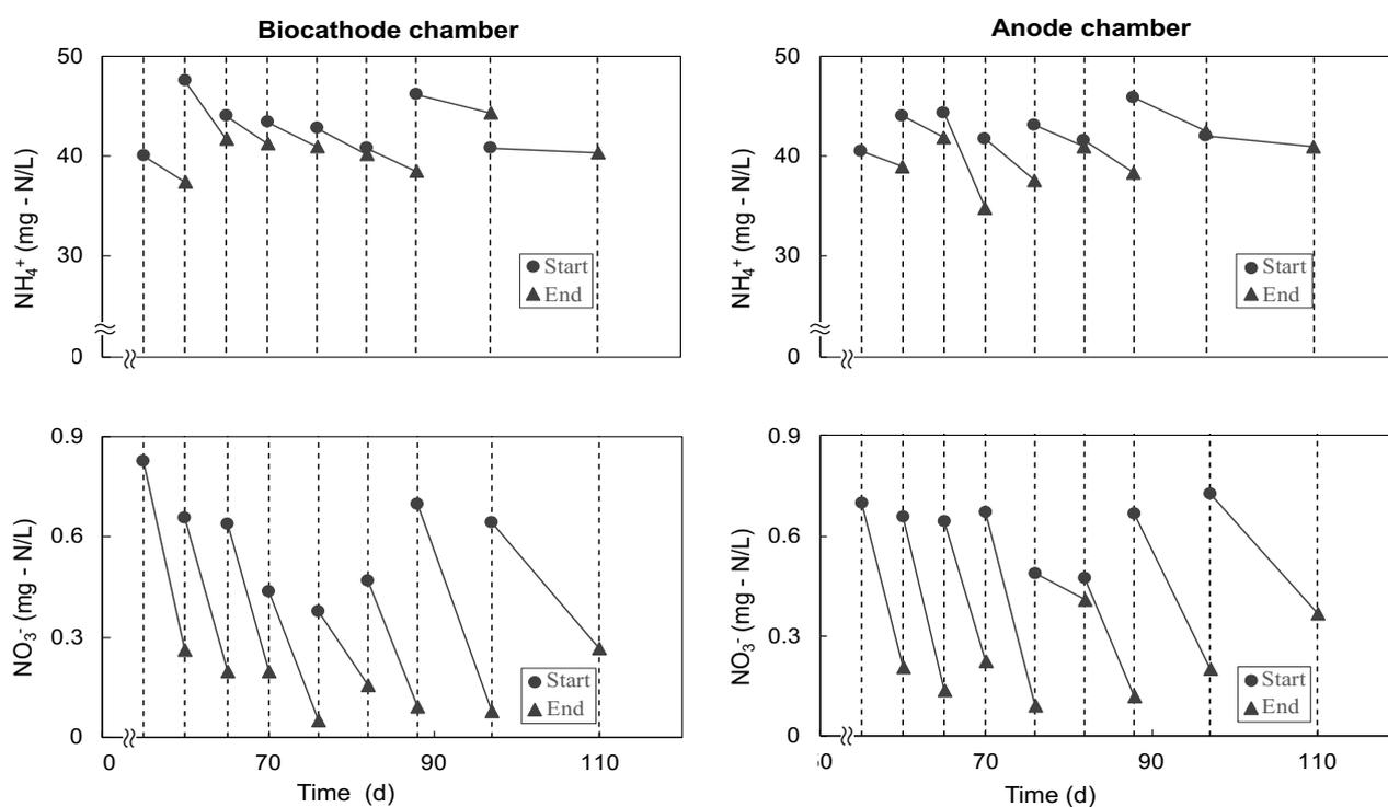
Fig. 3-5  $\text{NH}_4^+$ -N and  $\text{NO}_3^-$ -N at the start and end of each batch operation.
