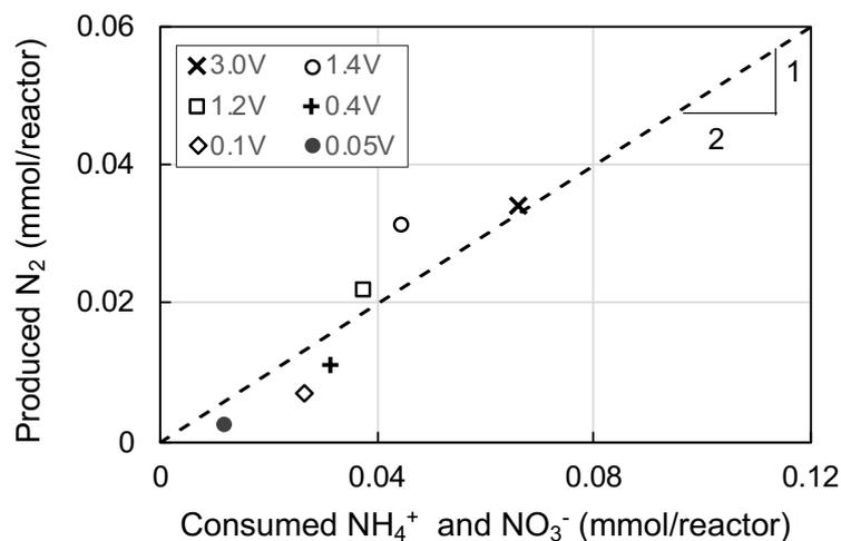
**Fig. 3-6** Relationship between the produced  $\text{N}_2$  and total amount of consumed  $\text{NH}_4^+$  and  $\text{NO}_3^-$ .
