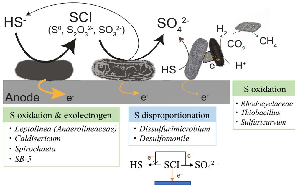
**Fig. 5-13** Proposed pathways of the sulfide oxidation at the bioanode
