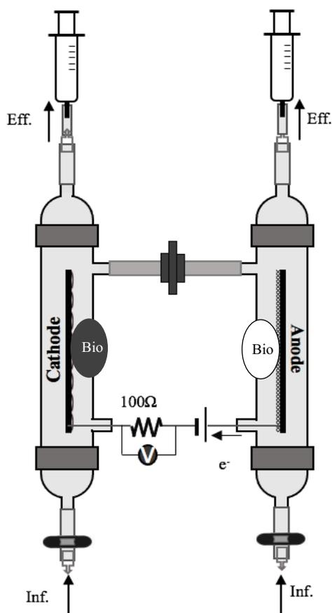
**Fig. 5-1** Schematic representation of microbial electrosynthesis system consisting of two chambers connected with a cation exchange membrane (MES; biotic anode).
