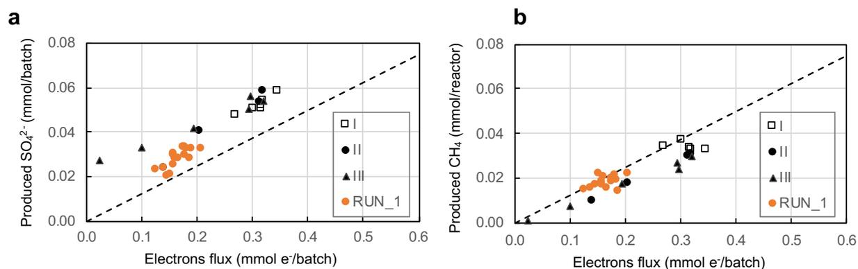
**Fig. 5-9** Produced SO<sub>4</sub><sup>2-</sup> and CH<sub>4</sub> versus electron flux  $N_e$ . Dash line: theoretical production based on the half reactions.
