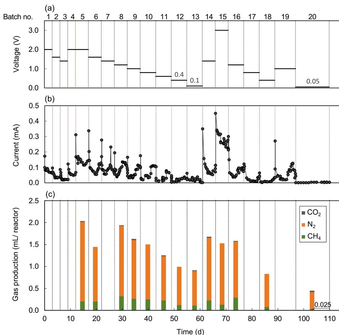
**Fig. 3-4** Time courses of applied voltage (a), current (b), and gases (CH<sub>4</sub>, N<sub>2</sub>, and CO<sub>2</sub>) produced (c) in batch experiments
