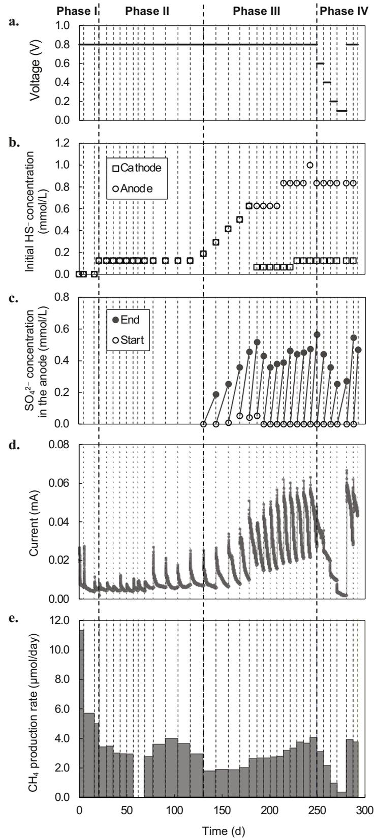
**Fig. 4-2** Time courses of (a) applied voltage, (b) initial HS<sup>-</sup> concentration, (c) SO<sub>4</sub><sup>2-</sup> concentration in the anode, (d) current, and (e) CH<sub>4</sub> production rate in batch experiments.
