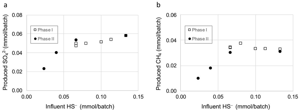
**Fig. 5-7** Relationship between the produced SO<sub>4</sub><sup>2-</sup> (a), CH<sub>4</sub> (b) and influent HS<sup>-</sup>
