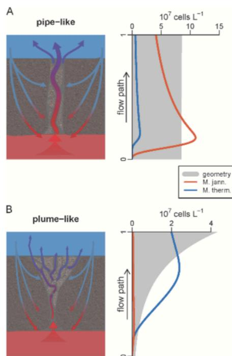
**Fig. 2-3** General reactive transport model results for straight-pipe (a) and expanding-plume (b) models. Lateral cross-sections depicting each model are shown on the left. The estimated concentration of *M. jannaschii* and *M. thermolithotrophicus* cells and the geometry of the flow path are shown on the right. The fluid temperatures at steps 0 and 1 are 84.6 and 26.7 °C, respectively
