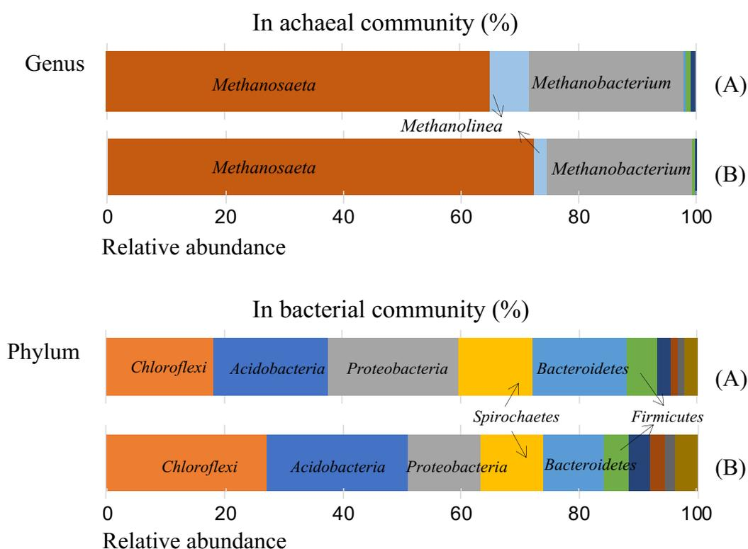
**Fig. 5-10** Comparison between two microbial communities (A) and (B) based on 16S rRNA gene. (A) : microbial community developed at the biocathode in chapter 4
