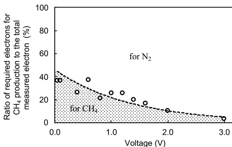
**Fig. 3-10** Relationship between the ratio of required electrons for CH<sub>4</sub> production to total measured electrons  $N_e$  and applied voltage.
