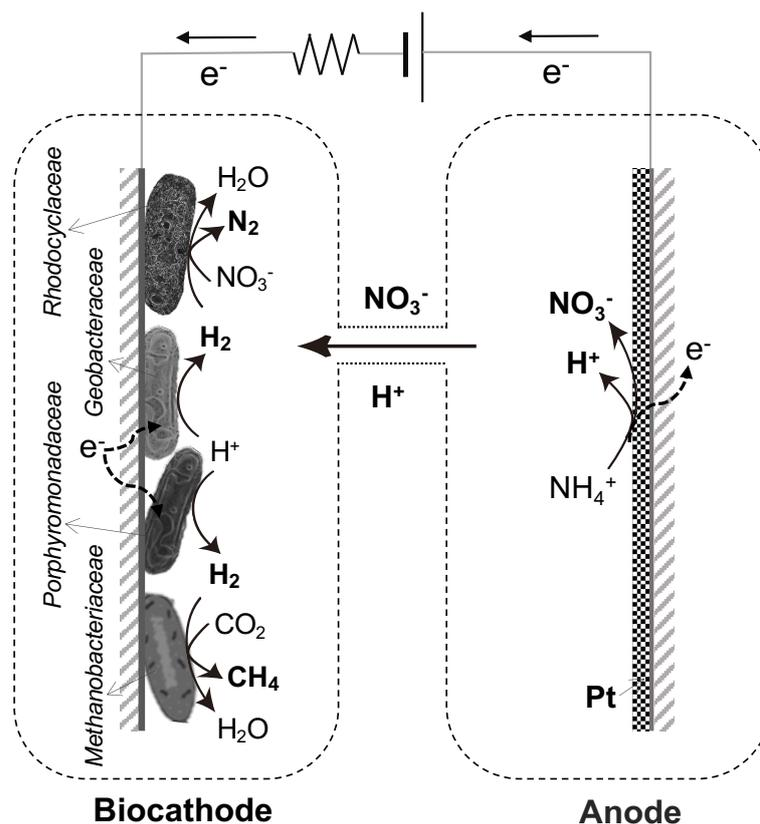
**Fig. 3-12** Scheme of electronic methane and nitrogen production in MEC reactor without organic substances.
