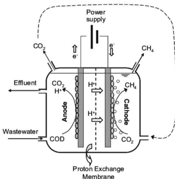
**Fig. 2-7** Schematic drawing of a bioelectrochemical system for wastewater treatment and simultaneous CH<sub>4</sub> production based on bioelectrochemical CO<sub>2</sub> reduction
