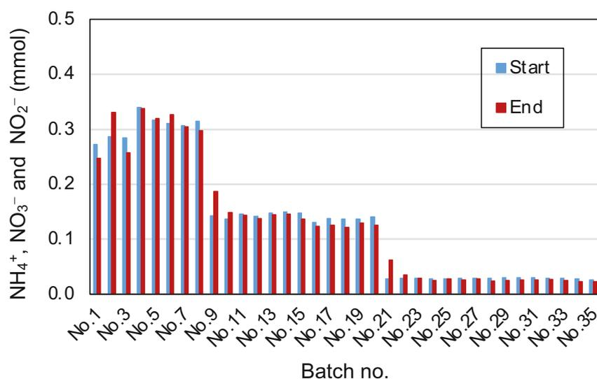
**Fig. 4-4** Total amount of  $\text{NH}_4^+$ ,  $\text{NO}_3^-$  and  $\text{NO}_2^-$  in both chambers at the start and end of each batch experiment.
