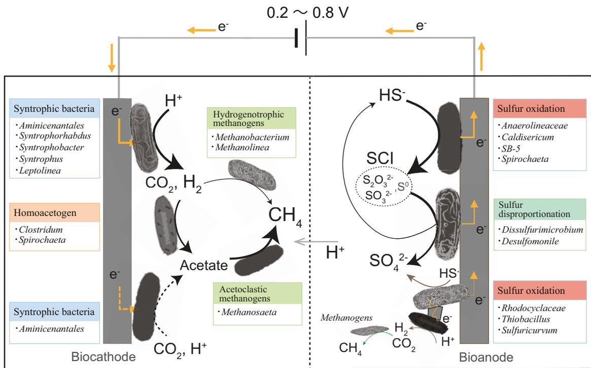
**Fig. 5-14** Coupling of CO<sub>2</sub> reduction at the biocathode and sulfur oxidation at the bioanode with the assistance of microbial catalyst in microbial electro-synthesis system
