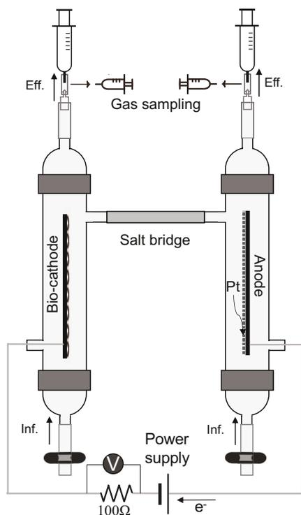
**Fig. 3-1** Schematic of MES consisting of two chambers connected with a salt bridge.
