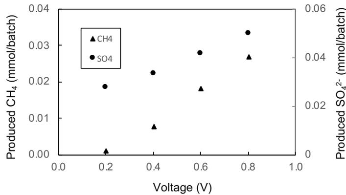
**Fig. 5-8** Produced CH<sub>4</sub> and SO<sub>4</sub><sup>2-</sup> at different applied voltage in phase III (RUN 3.2)
