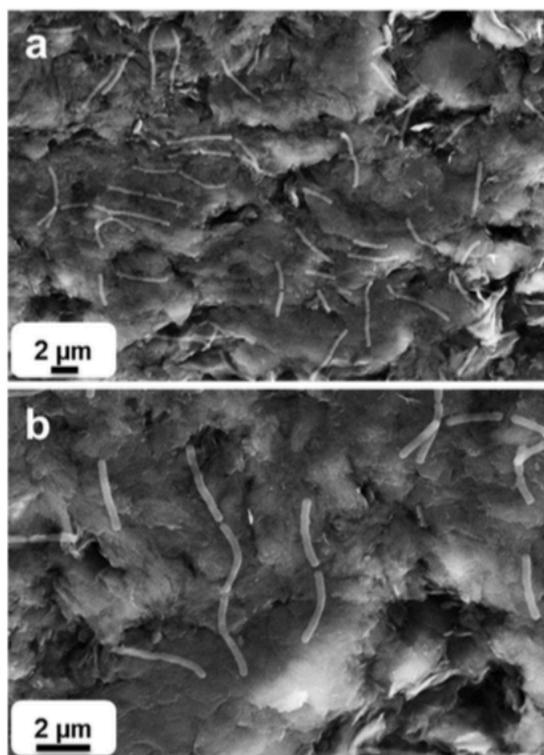
**Fig. 2-5** Scanning electron micrographs of strain IM1. Cells of strain IM1 attached to a graphite surface that served as the sole electron donor for microbial electrosynthesis of methane. Scanning electron micrographs shown in (a) 5000× and (b) 10,000× magnification. (Beese-Vasbender *et al.*, 2015)
