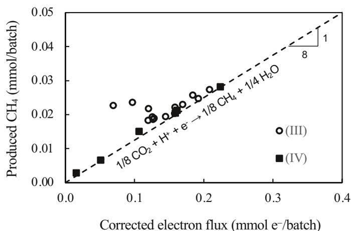
**Fig. 4-10** Relationship between the produced methane and corrected electron flux to assess the influence of abiotic current.
