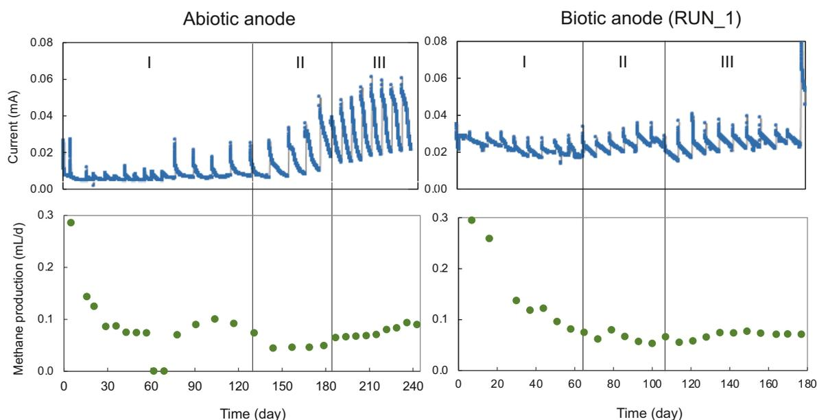
**Fig. 5-5** Comparison with the current and methane production of batch experiments using Pt-catalyst (abiotic anode)
