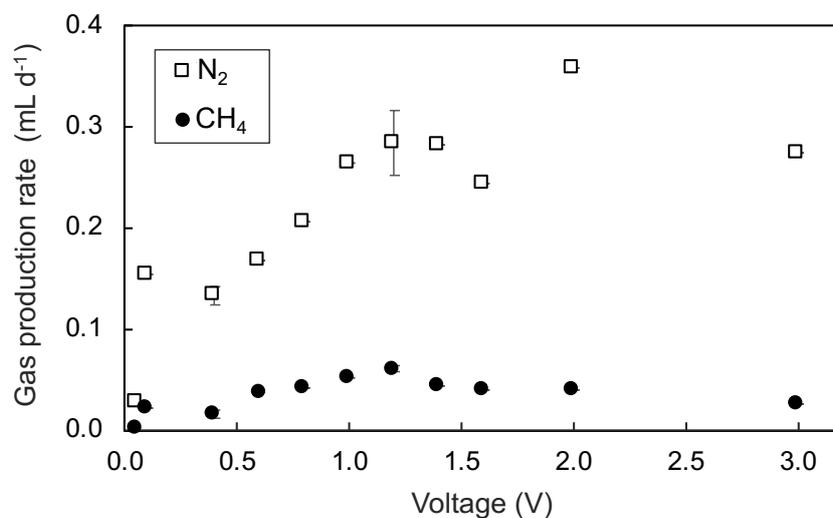
**Fig. 3-7** Gas production rates at different applied voltages
