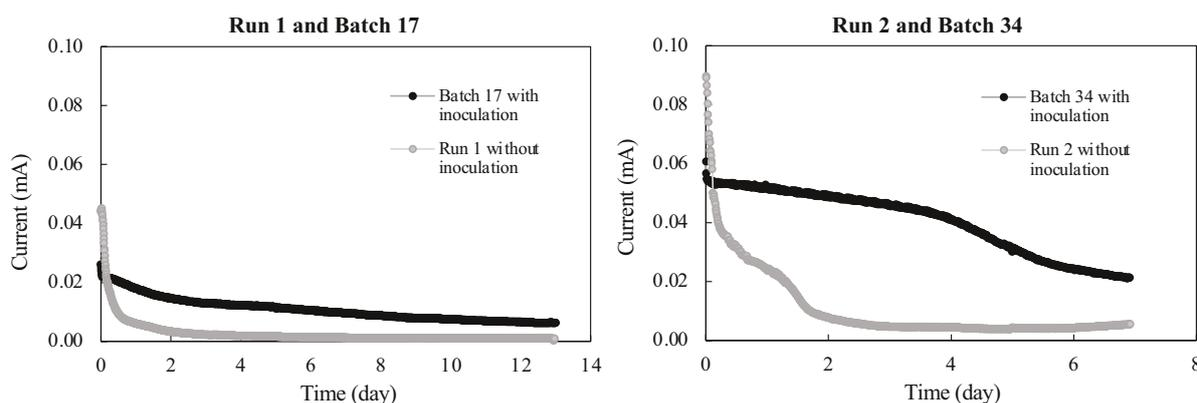
**Fig. 4-9** Time courses of current in batch experiments under abiotic and biotic conditions**Table 4-4** Electron flux and the ratio of abiotic to biotic flux
