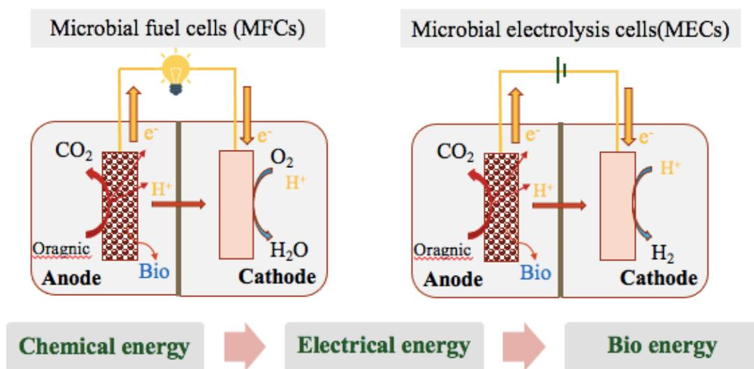
Fig. 2-6 Scheme of microbial fuel cell and microbial electrolysis fuels
