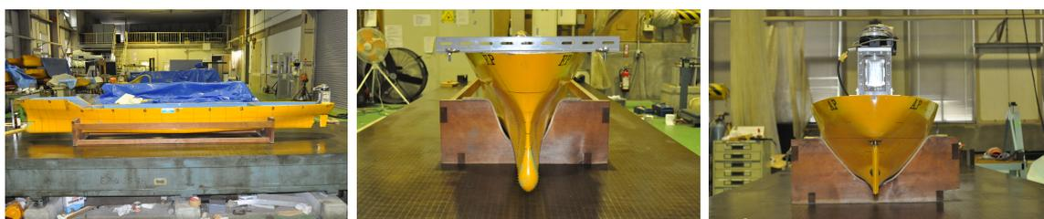
Fig. 3.2: Side, front and rear views of towed ship model (SR108)
