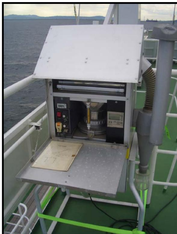
**Figure 3-2.** High Volume Air Sampler set up on the deck of Toyoshio Maru
