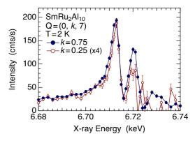
FIG. 6. (Color online) X-ray energy dependencies of the magnetic Bragg peak at  $\mathbf{Q} = (0,0.75,7)$  and (0,0.25,7) at 2 K without polarization analysis after subtracting the background and being corrected for absorption. The data for k = 0.25 are multiplied by four. The error bars represent only the statistical error.
