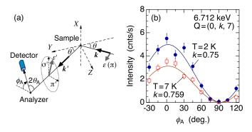
FIG. 9. (Color online) (a) Scattering geometry of the experiment with polarization analysis. Cu-200 reflection is used as an analyzer, where  $2\theta_A = 92.55^{\circ}$  at 6.712 keV. (b)  $\phi_A$  dependence of the resonant intensity at 6.712 keV (E2). Solid line is a fit to the data assuming a purely  $\pi$ - $\sigma'$  scattering.
