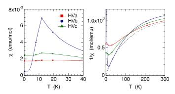
FIG. 11. (Color online) Calculated temperature dependencies of magnetic susceptibility and inverse magnetic susceptibility using a mean-field model and crystal-field parameters described in the text. The dot-dashed curve shows  $1/\chi$  for a free Sm<sup>3+</sup> ion with J=5/2 ground state and J=7/2 excited state at 1500 K.
