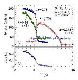
FIG. 8. (Color online) (a) Temperature dependencies of the magnetic Bragg peak intensities at the first and third harmonic positions and at 6.712 keV. The intensities of the third harmonic peaks are multiplied by three. (b) The ratio of the third harmonic intensity to the first harmonic intensity as a function of temperature after subtraction of the background. The solid line is a guide for the eye.
