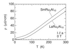
FIG. 1. Temperature dependence of the resistivity of  $SmRu_2Al_{10}$  and  $LaRu_2Al_{10}$  at zero field.
