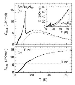
FIG. 4. (a) Temperature dependence of the magnetic specific heat obtained after subtracting the specific heat of  $LaRu_2Al_{10}$ . The inset shows the raw data of specific heat of  $SmRu_2Al_{10}$  and  $LaRu_2Al_{10}$ . The dashed line shows a calculation of the Schottky-type specific heat obtained by assuming a CEF Hamiltonian with a level scheme of 0 K–47 K–95 K. (b) Temperature dependence of the magnetic entropy.
