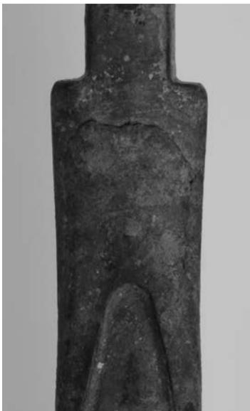
**Figure 3. Crack in guard
