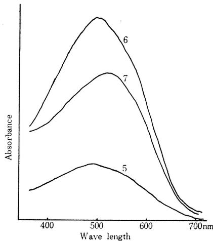
Fig. 4. Absorption spectra of unknown fractions (Fraction 5, 6 and 7) in petroleum ether.
