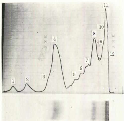
Fig. 1. Photograph of thin-layer chromatogram and its densitometry of carotenoids obtained from the exoskeleton of crayfish. *n*-hexane, ethylacetate (85 : 15).
