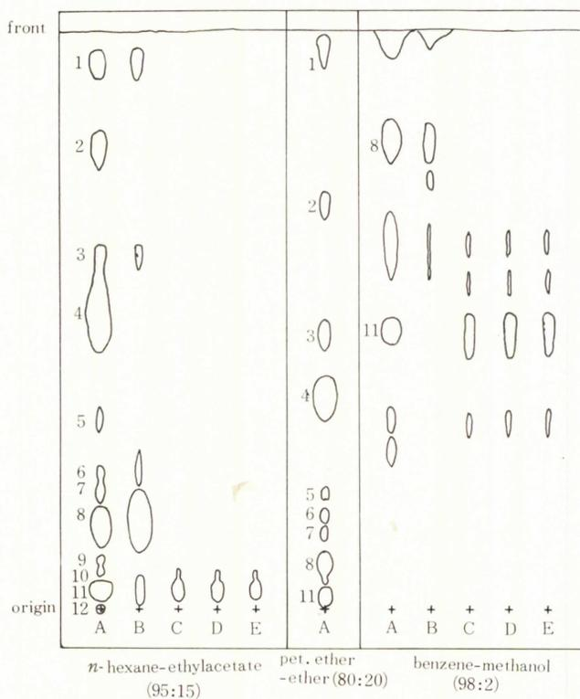
Fig. 2. Schematic chromatograms of carotenoids on silica gel plates.
