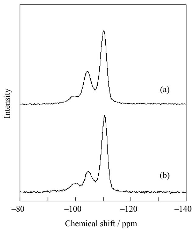
Fig. 4  $^{29}\text{Si}$  MAS NMR spectra of CHA type zeolites obtained (a) without seed crystals (sample no. 1) and (b) with seed crystals (sample no. 5).
