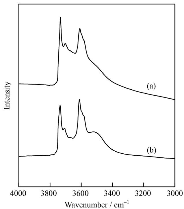
Fig. 5 FT-IR spectra of H-CHA type zeolites. (a) CHA type zeolite obtained with seed crystals in the presence of NaCl (sample no. 5) and (b) Na<sup>+</sup> cation-free CHA type zeolite obtained with seed crystals (sample no. 15).
