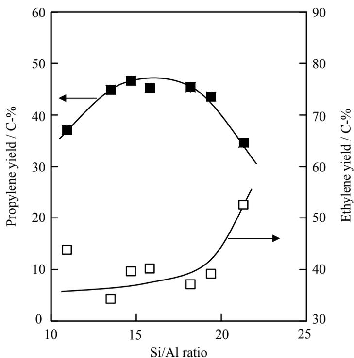
Fig. 7 Relationship between Si/Al ratio of CHA type zeolite and yield of light olefins ((□) ethylene and (■) propylene). Reaction conditions: temp. = 400 °C, W/F = 0.0125 g min mL<sup>-1</sup>.
