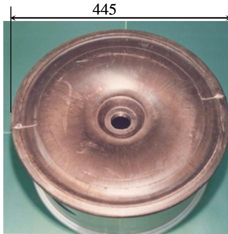
**Fig.2.27** Photograph of as-forged wheel
