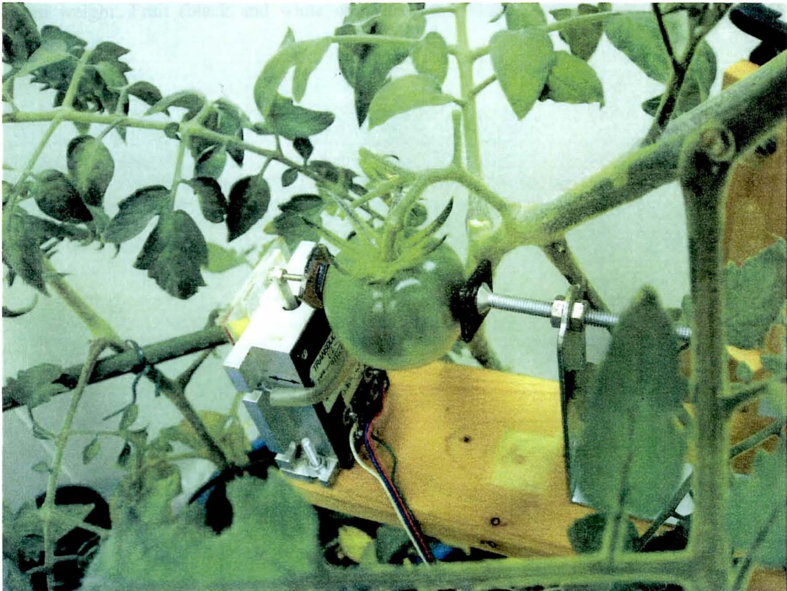
Fig.1. Tomato fruit diameter was measured using a shrinkage type micro-displacement detector.
