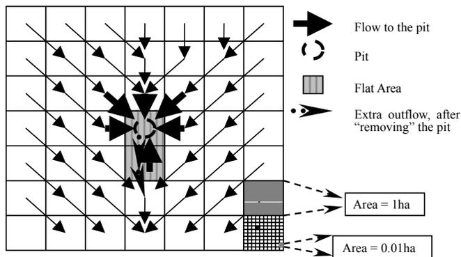
**Figure 2:** Schematic representation of the Flood-Routing Algorithm to remove a “pit”. The pit area is eliminated by modifying the height of the cell, in order to match it with those who surround it and make the area “FLAT”.
