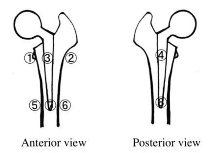
Fig. 4. Sites of attachment of strain gauges.
