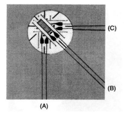
Fig. 3. Strain gauge; gauge element a (A), gauge element b (B), gauge element c (C)
