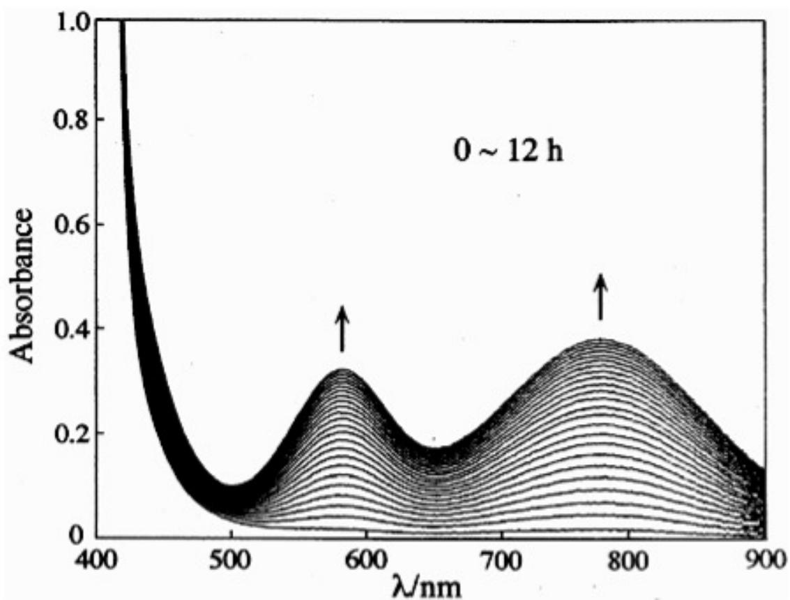
Fig. 4. Successive absorption spectra observed at 30 min intervals for 12 h under anaerobic conditions. A Tris-HCl buffer solution at pH 7.0 containing 20mM of  $\text{Na}_3[\text{VO}_2(\text{EDTA})]$  and 200 mM of NADPH was used. See [54].
