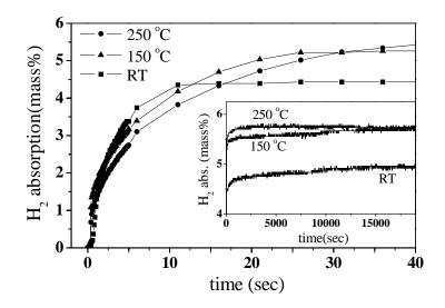
Figure 1. The amount of hydrogen absorption as a function of reaction time for the catalyzed Mg at room temperature RT (~20 °C), 150 °C and 250 °C under 1 MPa hydrogen.
