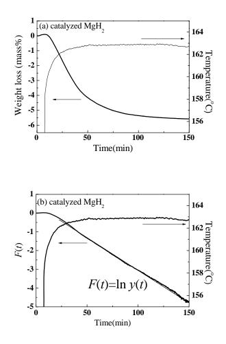
Figure 2. (a) Weight loss due to H-desorption and the aspect of temperature fluctuation around fixed temperatures as a function of H-desorption reaction time and (b) normalized hydrogen concentration function F(t), and the aspect of temperature fluctuation around fixed temperatures as a function of H-desorption reaction time for the catalyzed MgH<sub>2</sub>.
