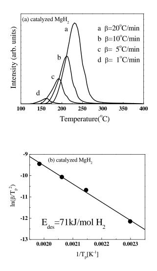
Figure 3. (a) TDMS of hydrogen under various heating rates ( $\beta$ =1,5,10,20 °C/min) from the catalyzed MgH<sub>2</sub> The intensities of longitudinal axis indicates the amount of hydrogen desorption per unit time. (b) Kissinger plots for the hydrogen desorption reaction for the catalyzed MgH<sub>2</sub>. Notations:  $T_p$  indicates the peak temperatures in thermal desorption spectra.
