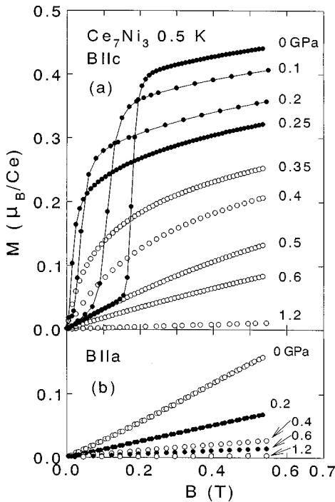
FIG. 1. Isothermal magnetization curves of  $\text{Ce}_7\text{Ni}_3$  at 0.5 K for  $B \parallel c$  and  $B \parallel a$  under various pressures.
