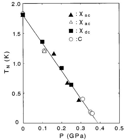
FIG. 5. Pressure dependence of the magnetic transition temperature  $T_N$  for  $\text{Ce}_7\text{Ni}_3$  determined by the measurements of ac [▲ (Ref. 12), △] and dc susceptibility (■) and specific heat (○).
