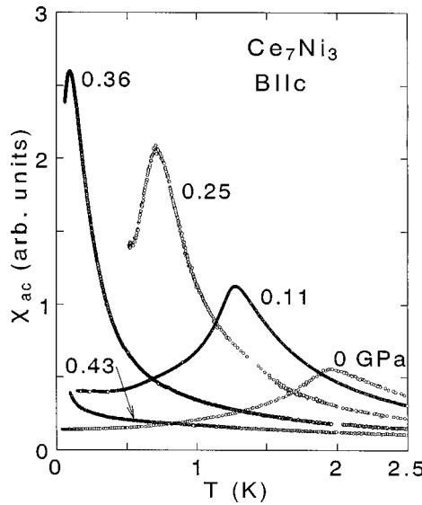
FIG. 3. Temperature dependence of  $\chi_{\text{ac}}$  of  $\text{Ce}_7\text{Ni}_3$  for  $B \parallel c$ . The data at 0.25 GPa represents  $\chi_{\text{dc}}(T)$ .
