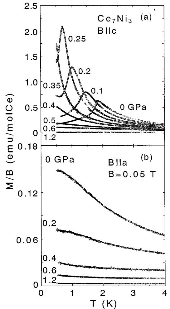
FIG. 2. Temperature dependence of the magnetic susceptibility  $M/B$  of  $\text{Ce}_7\text{Ni}_3$  for  $B \parallel c$  and  $B \parallel a$  under various pressures.
