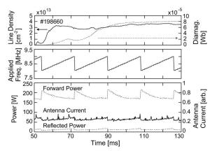
FIG. 4. The variation of the plasma and the transmitter parameters in a typical discharge. The frequency is swept in a staircase pattern since a certain length of the step width is required for the FFT analysis.
