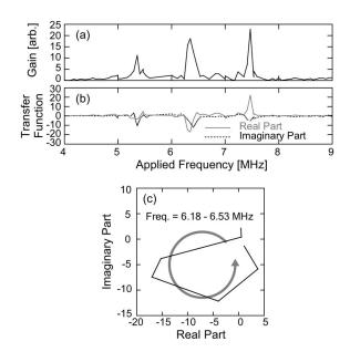
FIG. 5. (a) The gain-frequency diagram. The eigenmodelike discrete peaks are clearly observed at 5.35, 6.40, and 7.45 MHz. (b) The frequency dependence of the real and imaginary parts of the complex transfer function. (c) An example of the complex plane representation for the fourth peak near 6.4 MHz. The trajectory is approximately a circle, which indicates the resonant excitation of an eigenmode.
