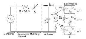
FIG. 3. A simple circuit model of the antenna-eigenmodes coupling. Each eigenmode can be represented by a RLC resonance circuit.  $R_{pi}$ ,  $L_{pi}$ , and  $C_{pi}$  are the resistance, inductance, and capacitance of the *i*th eigenmode in the plasma.  $M_i$  is the mutual inductance between the antenna and the eigenmodes.
