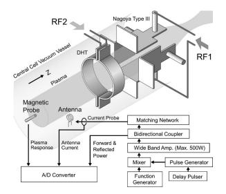
FIG. 2. The schematic diagram of the rf probe system.
