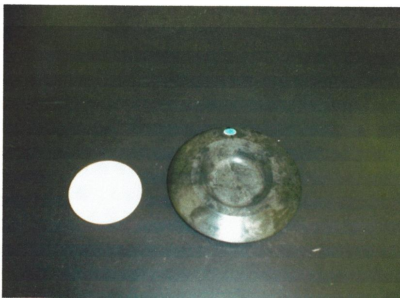
Fig.1-10 Ceramic Cell (left)、Open Cup (B+L K.K)(right)
