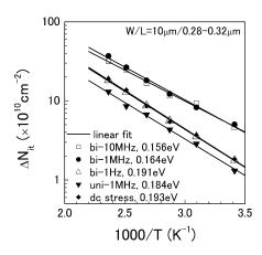
Fig. 4. Temperature dependence of  $\Delta N_{\rm it}$  at five typical stress configurations. Devices with L = 0.28–0.32  $\mu$ m, stressed for 10<sup>3</sup> s at  $V_a$  = 2.9 V except that  $V_a$  = 2.6 V for 10-MHz bipolar stress to avoid.  $\Delta N_{\rm it}$  saturation. The activation energy E<sub>a</sub> was extracted from the linear fitting of these Arrhenius plots.
