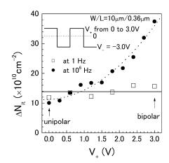
Fig. 2. Interface trap generation  $\Delta N_{\rm it}$  under unsymmetrical bipolar BT stress as a function of  $V^+$  at 1 and 10<sup>6</sup> Hz.  $V^-$  is fixed to -3.0 V. Devices with L = 0.36  $\mu$ m, stressed at 125 °C for 10<sup>3</sup> s. Inset is a schematic waveform applied on the gate.
