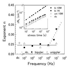
Fig. 3. Exponent *n* of the  $\Delta N_{\rm it}$  time power function as a function of stress frequency at unipolar and bipolar pulsed stresses. The data of dc stress is also given for comparison. Inset is the time evolution of  $\Delta N_{\rm it}$  for four typical stresses. The exponent n was extracted from the linear fitting of these plots.
