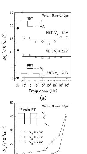
Fig. 1. Interface trap generation  $\Delta N_{\rm it}$  as a function of stress frequency at different stress voltage  $V_{\rm stress}$ , under (a) unipolar pulsed stress (L =  $0.40 \,\mu$ m), (b) bipolar pulsed stress (L =  $0.44 \,\mu$ m). Stressed at 125 °C for  $10^3$  s. The data of dc stresses are also shown for comparison, whose nominal stress time is 500 s. Inset is a schematic waveform applied on the gate.
