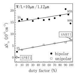
Fig. 2. Interface trap generation  $\Delta N_{\rm it}$  as a function of duty factor under unipolar and bipolar stresses with a square waveform of  $t_R=t_F=4.5$  ns and  $f=10^6{\rm Hz}$ . Devices have size of  $W/L=10~\mu{\rm m}/1.12~\mu{\rm m}$  and are stressed at 125 °C for  $10^3$  s. The 100% duty factor represents the dc negative BT stress (SNBTI), and the 0% duty factor represents the dc positive BT stress (SPBTI).
