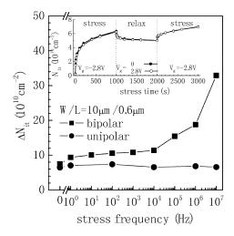
Fig. 1. Interface trap generation  $\Delta N_{\rm it}$  as a function of stress frequency under unipolar and bipolar BT stresses with a square waveform of  $t_R=t_F=4.5$  ns and duty factor of 50%. Devices have size of  $W/L=10~\mu{\rm m}/0.6~\mu{\rm m}$  and are stressed at 125 °C for  $10^3$  s. Inset is the time evolution of  $N_{\rm it}$  under stress-relax-stress sequence.
