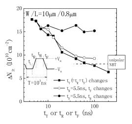
Fig. 3. Interface trap generation  $\Delta N_{\rm it}$  as a function of  $t_R$  (or  $t_F$ ) under bipolar stresses at  $10^6$  Hz with a trapezoidal waveform. Inset shows a schematic waveform to define  $t_L$ ,  $t_R$ ,  $t_H$  and  $t_F$ . Devices have size of  $W/L=10~\mu{\rm m}/0.8~\mu{\rm m}$  and are stressed at  $125~{\rm ^{\circ}C}$  for  $10^3$  s. For comparison,  $\Delta N_{\rm it}$  under unipolar stress with a square waveform ( $t_T=t_R=t_F=4.5~{\rm ns}$ ) is also shown.
