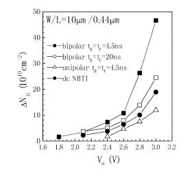
Fig. 4. Interface trap generation  $\Delta N_{\rm it}$  as a function of  $V_a$  under bipolar, unipolar and dc NBT stresses. Devices have size of W/L =  $10~\mu{\rm m}/0.44~\mu{\rm m}$  and are stressed at  $125~{\rm ^{\circ}C}$  for  $10^3$  s. The dynamic stress has a square waveform of  $f=10^6$  Hz, D=50%, and  $t_T=4.5$  ns or 20 ns.
